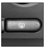
The lines you see on the rear window warm the glass. Press the button to start warming your window. A light will glow in the button while the defogger is working.
